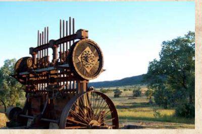
The All Nations gold mine (established 1860), is on the hill at the southern end of town. It was the last of the boom gold mines to close (in 1948). It developed into a large underground mine, operating at four levels in two shafts (the deepest being 100m). The ten-headed stamper battery remains.
